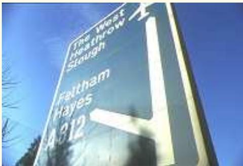
Indeed, the letters on a large motorway sign can be up to two feet (1200mm) high. These signs are on aluminium sheets, each panel 4ft square, rivetted to a backing frame.
