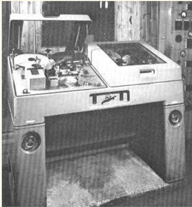
The film ran at 32cm/s. The overall amplitude-frequency characteristic: within  $\pm 2.5$  dB between 50 and 7000 Hz and within  $\pm 6$  dB between 30 and 8000 Hz with reference to the amplitude at 1000 Hz. Total distortion at 30 per cent modulation: 32 per cent at 60 Hz, 3.5 per cent at 1000 Hz, and 6.0 per cent at 4000 Hz. Noise: at least 50 dB below the output level at full modulation.
