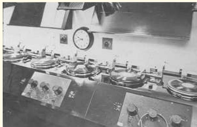
The picture above shows a bank of TD/7s in a radio studio, but the same equipment was used in the Dubbing Theatres, except that there was a shelf above the turntables to stack the, at times, large number of discs used in a dubbing session.
