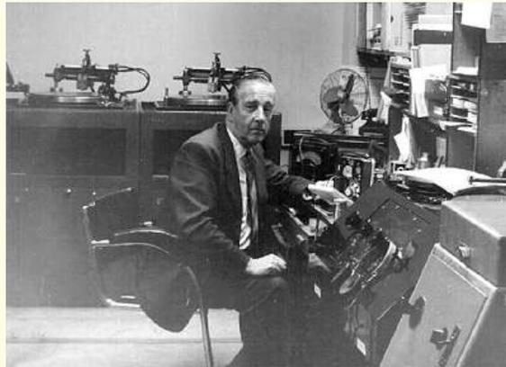
In the above picture, at the back are two Presto disk recorders. At the front, extreme right is the 3-speed LP player with, just alongside it, the twin turntable TD/7 replay unit (78rpm). [more](#)
