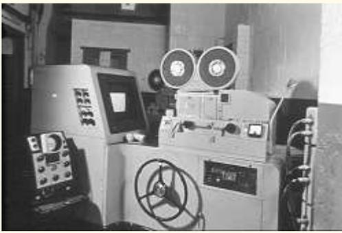
This telerecording system had been developed by BBC Research Department and installed at AP in CTR next to the Cintel telecine machines especially for the Coronation. They literally built themselves into a corner of CTR and with that breeze-block wall so close I don't know how they got around the machines.....
