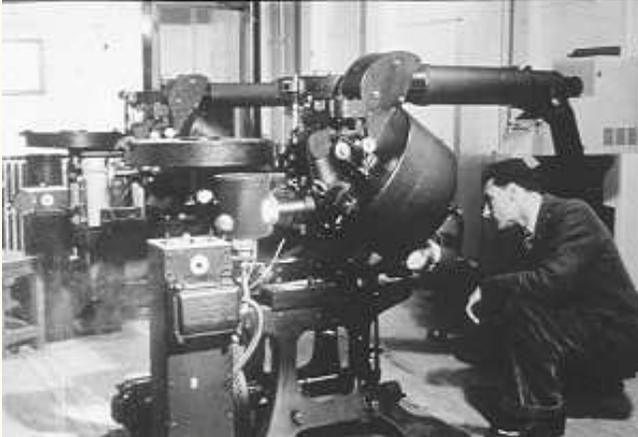
This is the pair of Mechau telecines used to show feature films from AP before the flying spot Cintel and EMI machines were developed. A 500w lamp illuminated the film and the continuous image looked into a standard Emitron camera.
