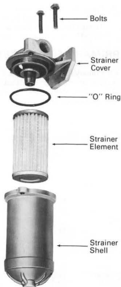
Fig. 1-4 - Fuel Suction Strainer, Exploded View
