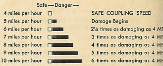
Damage to freight or car can be avoided by always keepin coupling speed within the safe range—NOT OVER 4 MILE PER HOUR—A BRISK WALK.
