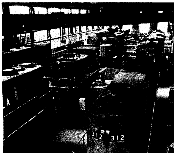
El Reno/ Locomotive shop has drop pits and all necessary tools to do any heavy repairs necessary, including changing main engines, generators or traction motors.
